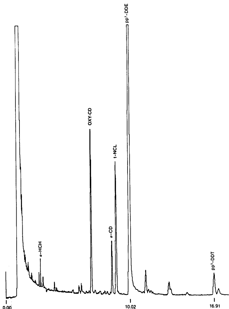
Figure 3. Typical 2nd-fraction chromatogram showing some of the organochlorine residues.
